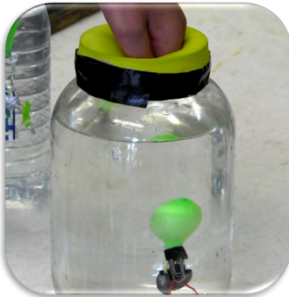
Figure 4: Cartesian diver; if you decrease the volume of the balloon and increase the pressure the diver will sink to the bottom. Much like a Buoyancy Compensation Device (BCD) allows a scuba diver to sink or float
