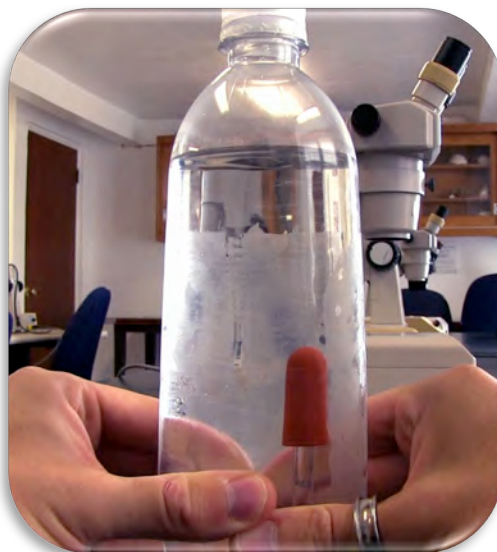
Figure 2: The increase in pressure decreases the volume of air in the pipette and this causes the pipette to sink
