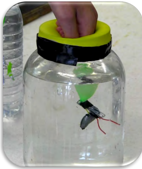
Figure 3: Cartesian diver at the surface; to make the diver sink you will need to decrease the volume of the balloon by increasing the pressure in the bottle
