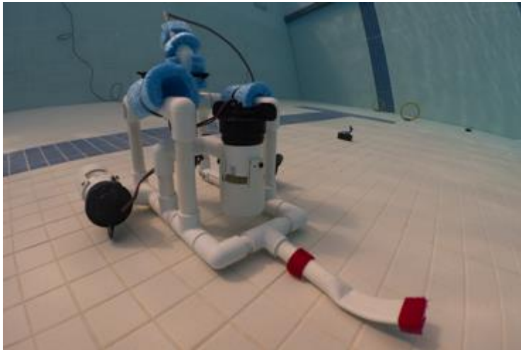
Figure 1: An example Beginner ROV, formed of the basic ROV kit with \frac{1}{2} " PVC only alongside floatation.
