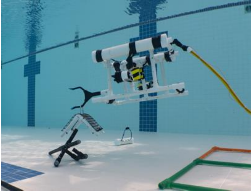
Figure 2: An example Beginner ROV that uses airtight ballast tanks in lieu of floatation for buoyancy. ROVs must pass safety inspection.
