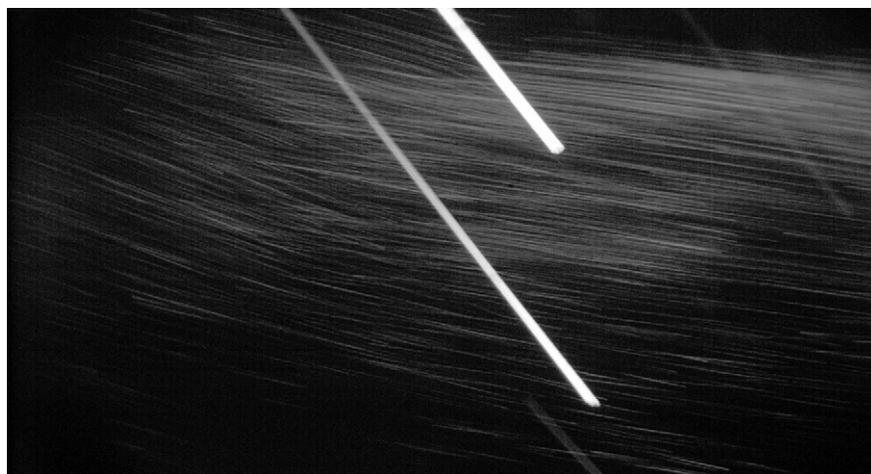
**Fig. 2.** High speed photograph of water droplets (the fine, nearly horizontal lines) being blown along with 200  $\mu\text{m}$  reference particles (the wide, more vertical lines).
